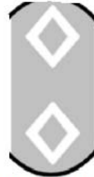
Diamond Marks Indicate A Crosswalk Ahead
